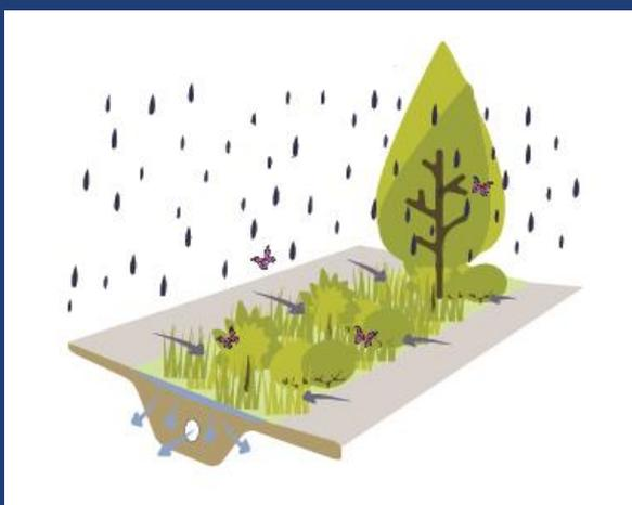
Sustainable drainage systems (SuDS) are a way of managing surface water. In cities and towns, they are used to slow the flow and contain surface water, mimicking the way that nature manages water, helping to reduce flooding and pollution.
